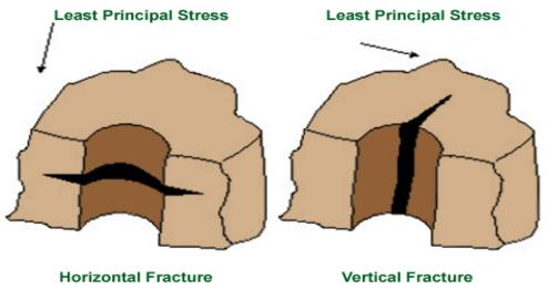
Figure 4: Diagram showing horizontal and vertical fractures in the direction of least principal stress [12]
