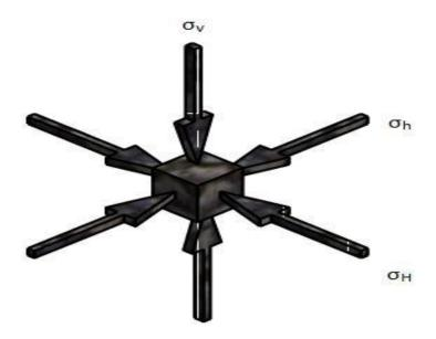
Figure 1: Orientation of In-situ stresses in a rock formation [6].
